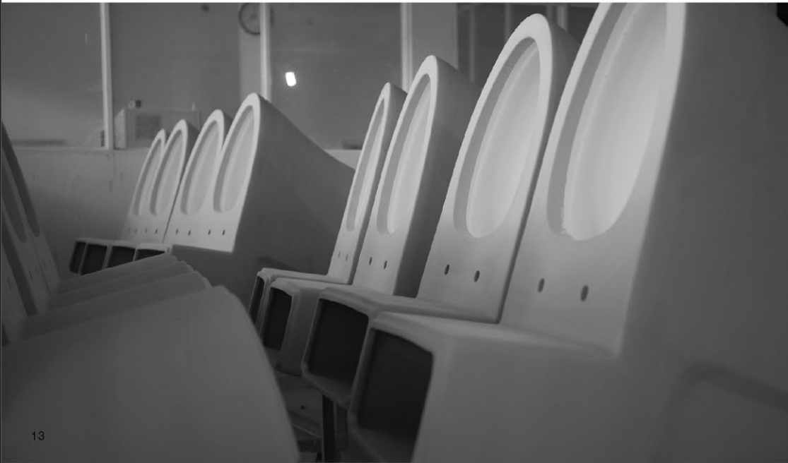
ABOVE: After demolded, FFC washbasins rest for slow drying
