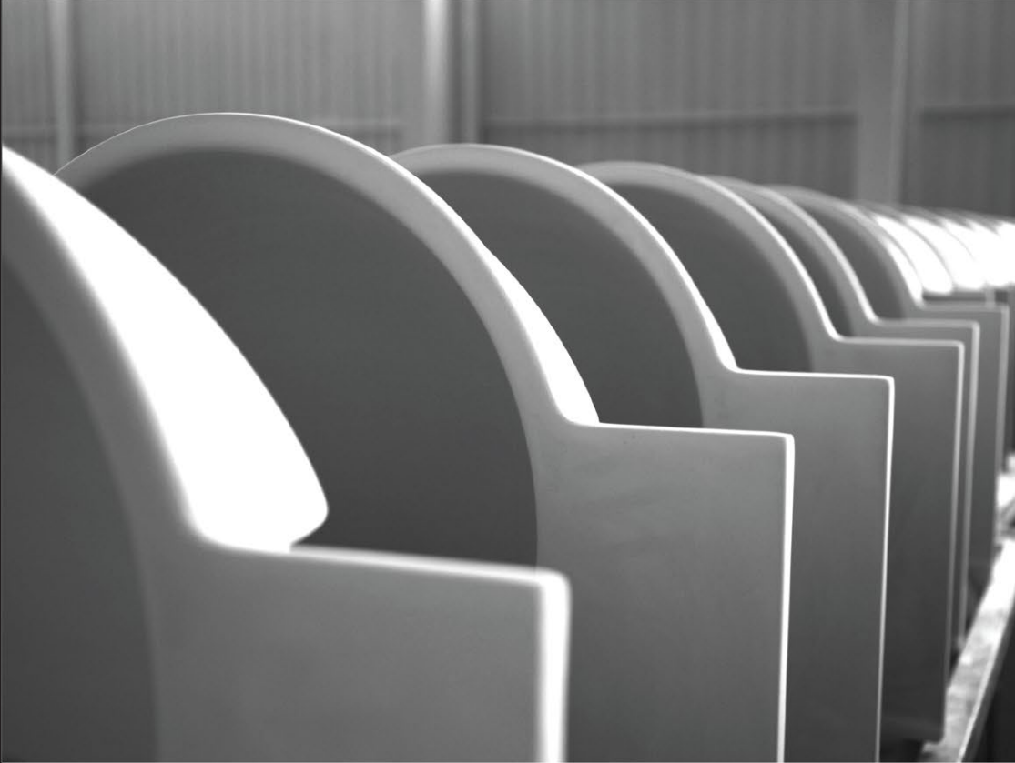
ABOVE: After demolded, FFC washbasins rest for slow drying
